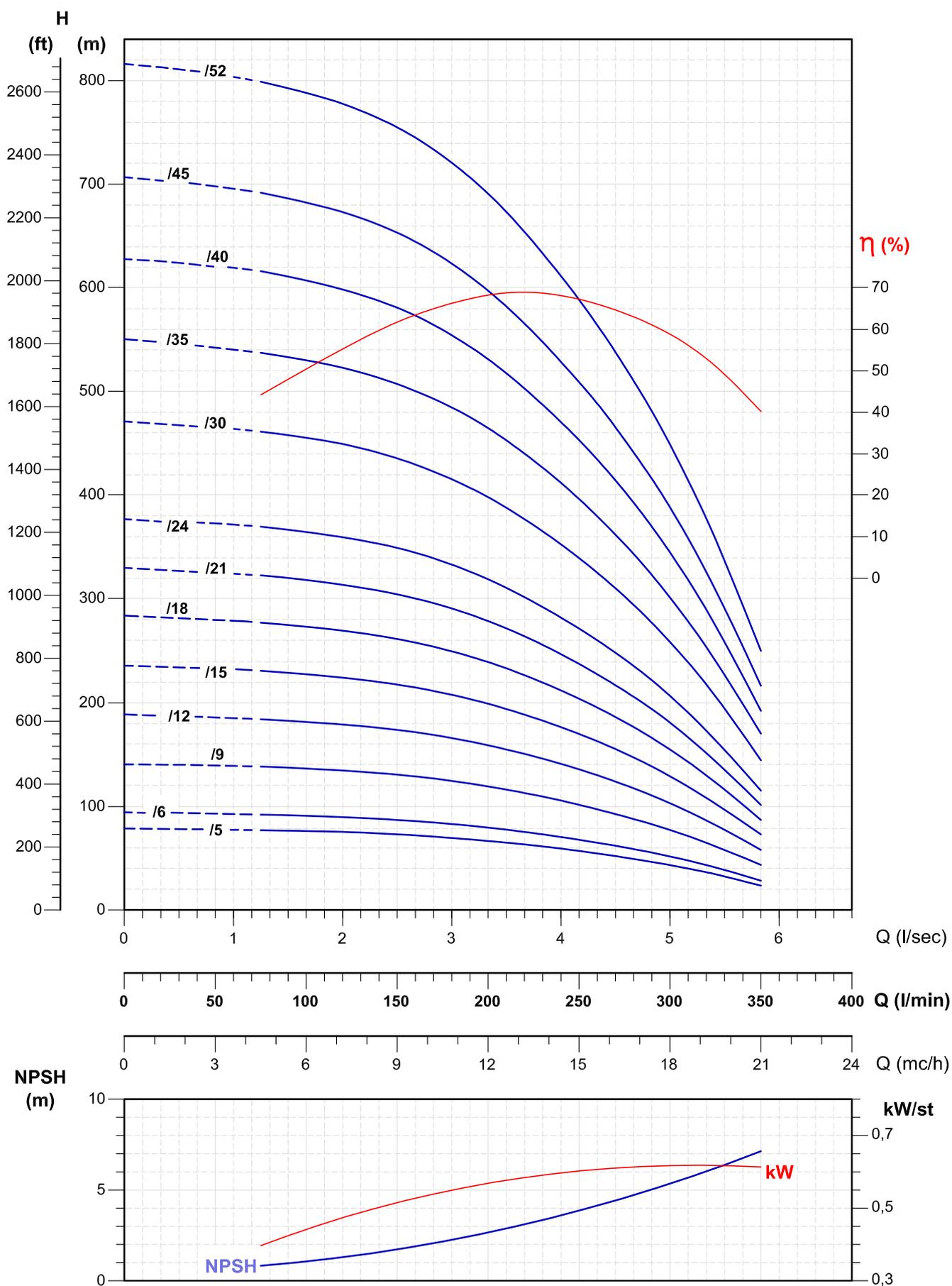
Tolleranze secondo EN ISO 9906 app.A Gr.2 - Tolerances according to EN ISO 9906 anx.A Gr.2 - Tolérances conformes EN ISO 9906 ann.A Gr.2
